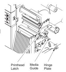
f. Pull the head leveling knob outward, and rotate it one detent. Rotating the knob clockwise from position 1 will adjust the printer for media that is narrower than the maximum width accepted by the printer. When the head leveling knob is rotated clockwise from the detent position just before position 1 to position 1, the printhead will return to the maximum media width position.
